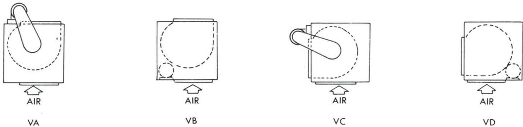
VERTICAL INVERTED CEILING, WALL AND FLOOR MODELS
